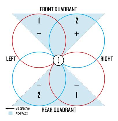
The front quadrant (pictured above) is the positive polarity stereo image, and the rear quadrant is the negative polarity stereo image. This distinction mirrors the difference in sound character when speaking into the front versus the rear of a mono bidirectional microphone. The waveform's polarity inversion turns what was initially a compression of air molecules into a rarefaction, and vice versa. Since music waves tend to be symmetrical, this difference is subtle.
