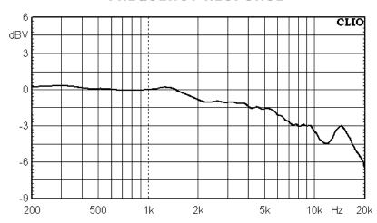
Data below 200 Hz omitted due to measuring room restrictions. 0 dVB is equivalent to 2.5 mV/Pa (-52 dBV) Normalized to 0 dB at 1kHz. 1/3 octave smoothing
